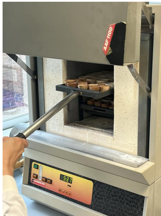
Figure 5b. Loss on ignition testing in the furnace.
